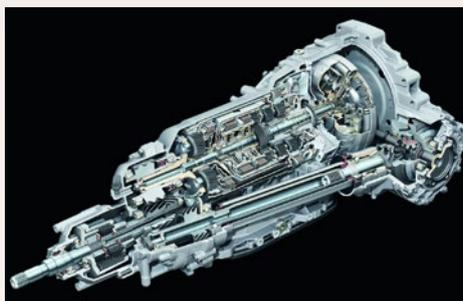
results in a power loss of around 8-10 per cent. Torque converters are, therefore, less fuel efficient than a manual gearbox or a CVT.
