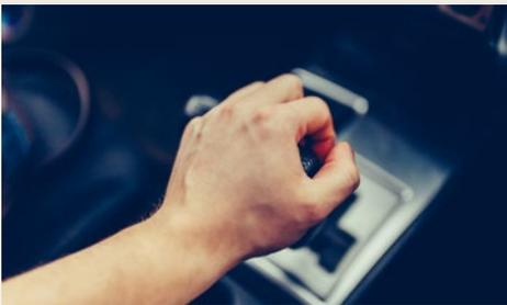
Some drivers tend to drive with one hand resting on the gear lever. This places weight on the transmission's bushings and synchronisers that leads to internal wear. Always keep both of your hands on the steering wheel and only take one hand off when you need to shift gears and place back on the steering wheel when you're done.
