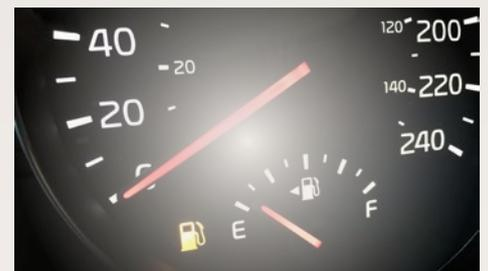
Modern cars use fuel pumps which are cooled by being submerged in fuel. But sometimes your budget may not be able to accommodate a full tank every time, leaving some drivers to fill small quantities at a time. It is always a good practice to keep at least a quarter of a tank of fuel at all times as lack of fuel in the reservoir can cause the pump to fail from overheating, leading to expensive repairs further down the road.
