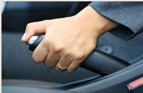
engage your handbrake. Some people leave their manual cars in gear, or in 'P' with automatic gearboxes. This puts weight on the cog or small piece of metal in the automatic gearbox which will eventually wear out and lead to complete failure over time. Using your handbrake along with it will reduce that stress on the components which are expensive to repair. A worn brake pad is easier to replace and costs much less.
